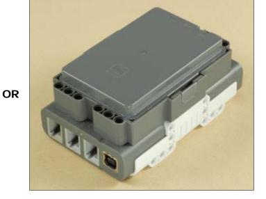
You can use the NXT with either AA batteries or the NXT Rechargeable Battery Pack.
