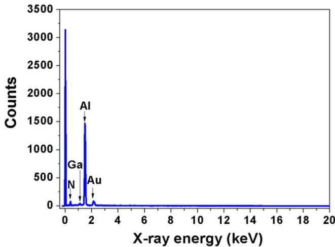
Figure 2. EDX spectrum of the AlN sample grown with Ga flow.
