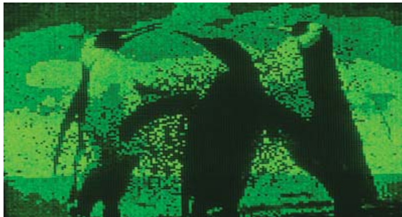
A grayscale projected image of penguins from a green InGaN microdisplay (having a pixel size of 12 \mu\text{m} , pitch distance of 15 \mu\text{m} , and 19,200 total pixels) operates at a driving current
