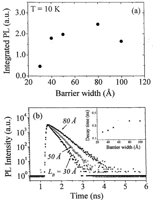
FIG. 3. (a) Integrated PL intensity of the well transition for the GaN/Al<sub>x</sub>Ga<sub>1-x</sub>N MQW samples as a function of  $L_B$  measured at 10 K. (b) The temporal responses of the well transitions in the GaN/Al<sub>x</sub>Ga<sub>1-x</sub>N MQW samples for various barrier widths at 10 K. The inset shows the barrier-width dependence of the decay lifetime for the well transition.
