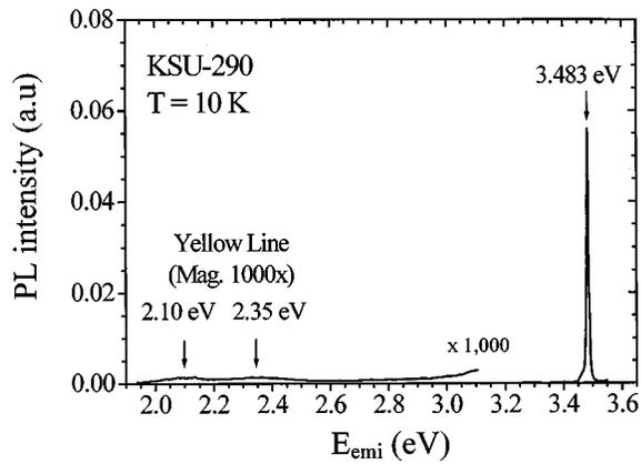
FIG. 1. Low-temperature PL spectrum for one of our undoped GaN epilayers (1.3  $\mu\text{m}$ ) recorded in a large emission energy scale to include yellow emission lines. The PL signal in the low-energy region ( $E < 3.1$  eV) has been magnified by a factor of 1000, indicating very little contribution from yellow emission and, hence, the high crystalline quality and purity of our samples.
