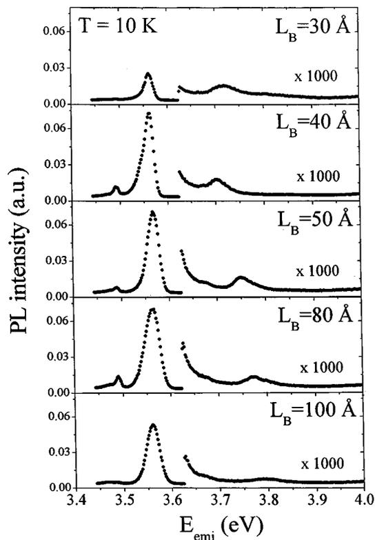
FIG. 2. cw PL spectra of a set of 30  $\text{\AA}$  well GaN/Al<sub>x</sub>Ga<sub>1-x</sub>N MQW samples with varying barrier widths,  $L_B = 30, 40, 50, 80,$  and  $100 \text{ \AA}$ , measured at 10 K. The MQW structures are grown under identical conditions.
