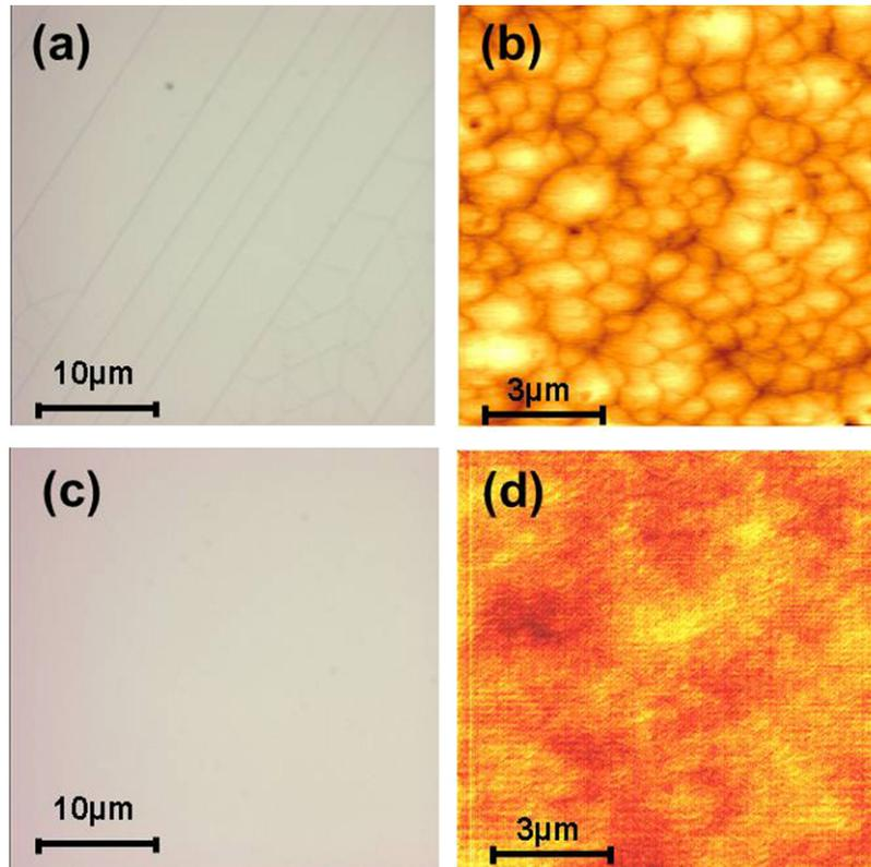
**Figure 1.** (a) A microscope image and (b) AFM image of AlN grown without Ga flow and (c) a microscope image and (d) AFM image of AlN grown with Ga flow.
