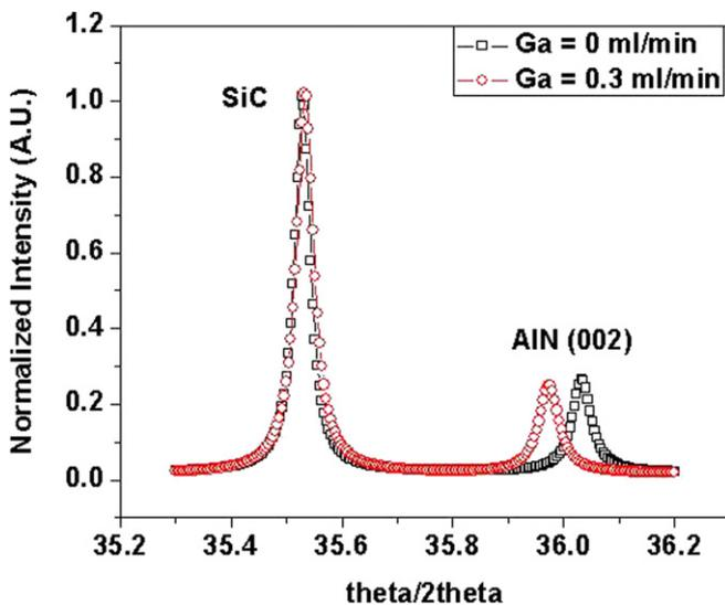
Figure 3. (002)  $\omega$ - $2\theta$  scans of the two AlN samples grown with and without Ga surfactant.
