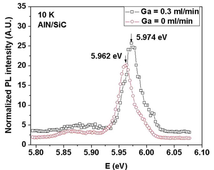
Figure 5. 10 K PL spectra of the two AlN samples grown with and without Ga surfactant, measured in a small spectral range from 5.8 to 6.1 eV.
