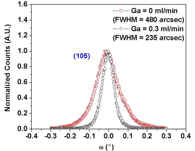
Figure 4. Rocking curves of the asymmetric (105) reflection peaks in AlN epilayers grown with and without Ga surfactant. FWHM is 235 arcsec for AlN sample with Ga surfactant and 475 arcsec for the AlN sample without Ga surfactant.
