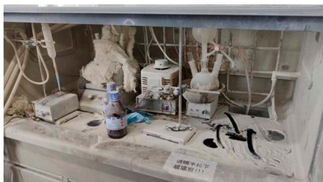
Figure 2. Accident scene after the fire was put out. The note at the front of the fume hood means "Please pull down the fume hood window."
