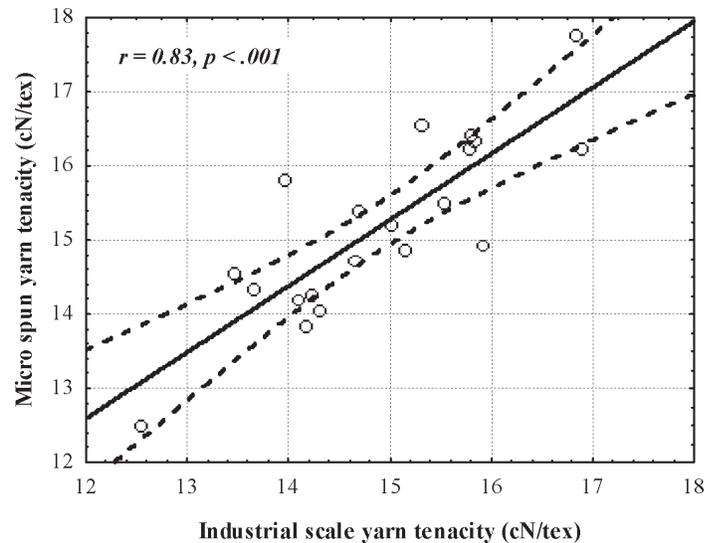
**Figure 3: Relationship between micro-spun and full-scale yarn strength**
