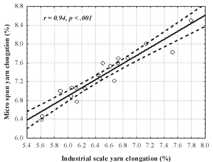
**Figure 4: Relationship between micro-spun and full-scale yarn elongation**
