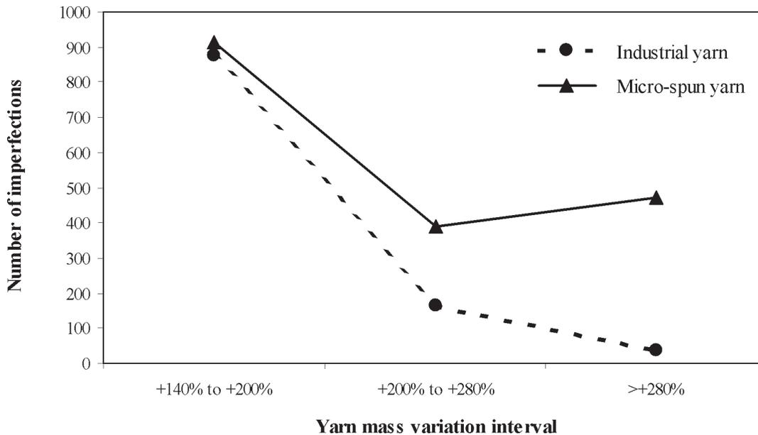
**Figure 7: Micro-spun and industrial yarn nep counts depending on the mass variation interval**
