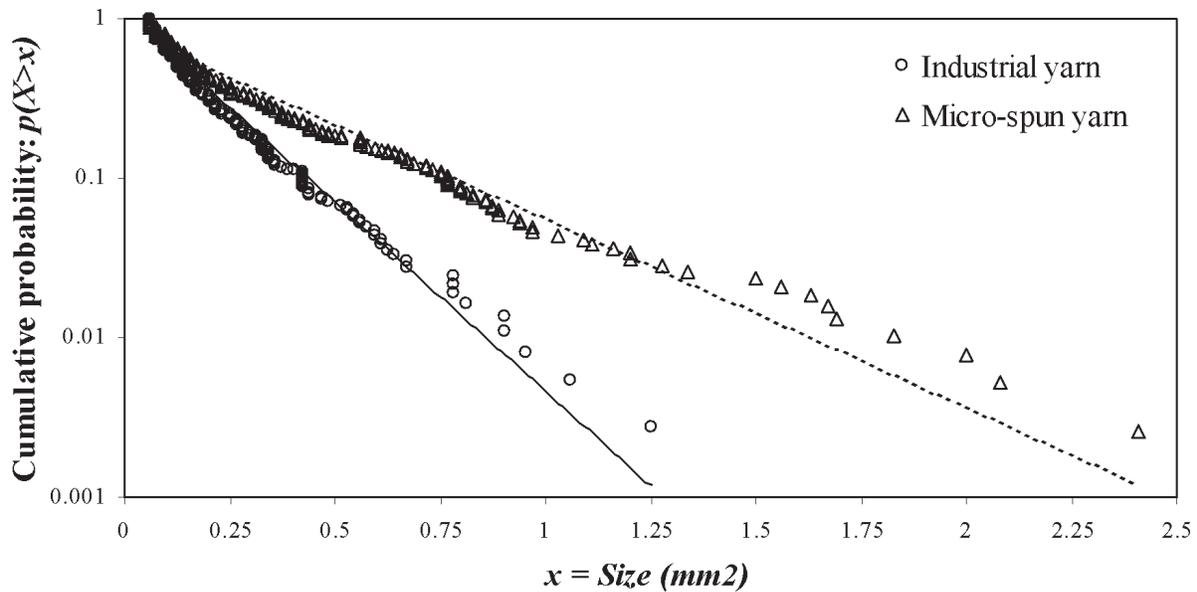
**Figure 9: Seed Coat Fragments size distribution for micro-spun and industrial yarns.**
