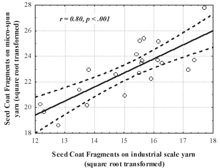
**Figure 8: Relationship between micro-spun and full-scale yarn Seed Coat Fragments**
