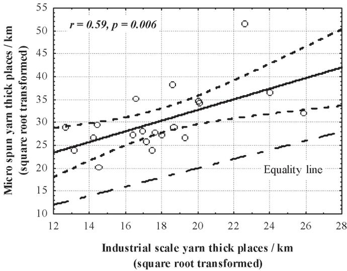
**Figure 5: Relationship between micro-spun and full-scale yarn thick places**
