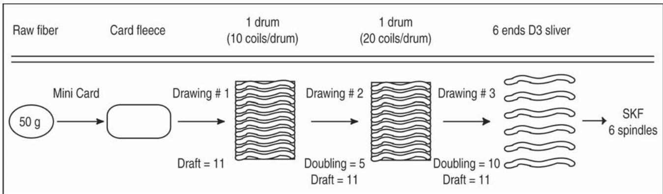
**Figure 2: Schematized micro-spinning operating protocol**
