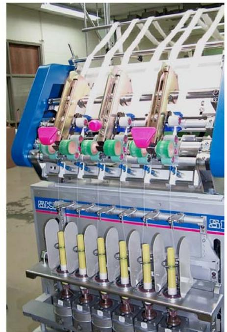
c) 6-spindle SKF Lab-Spinner
