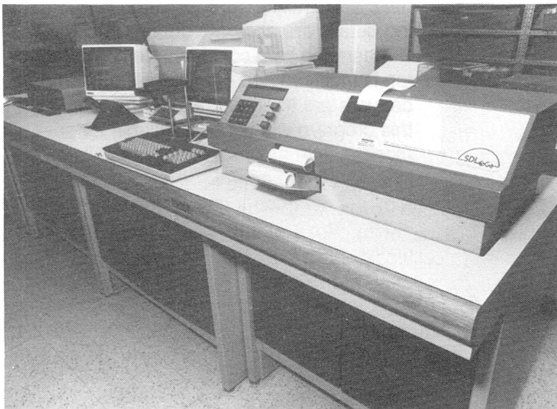
The Shirley FMT 3 has also been integrated with the Spinlab 900 HVI System, as seen in the photo at left
