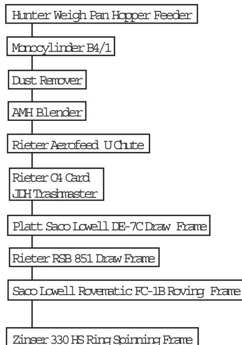
Figure 1: Processing Flow
