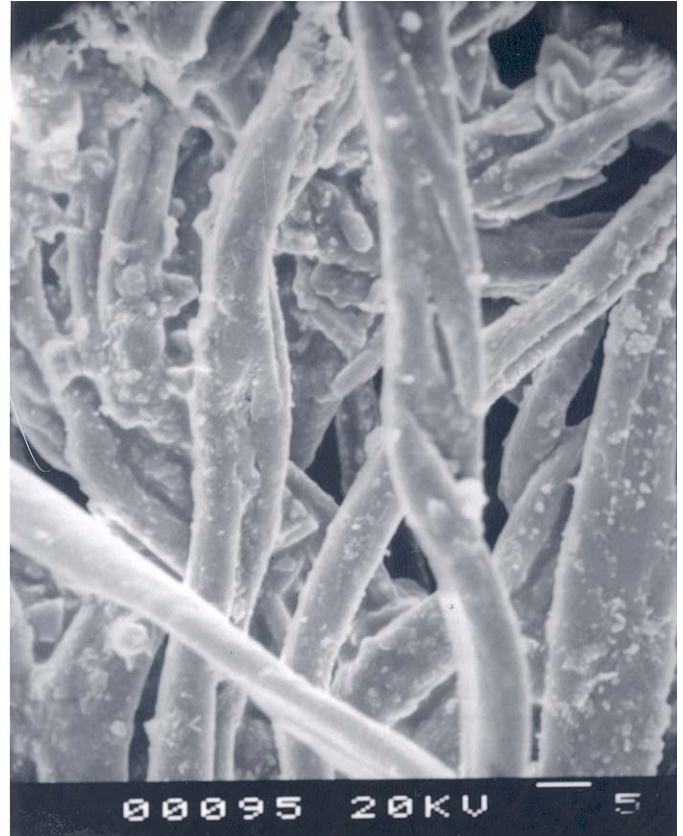
Figure 4: SEM micrograph of a yarn defect showing accumulation of other materials. Scale bar = 5 microns
