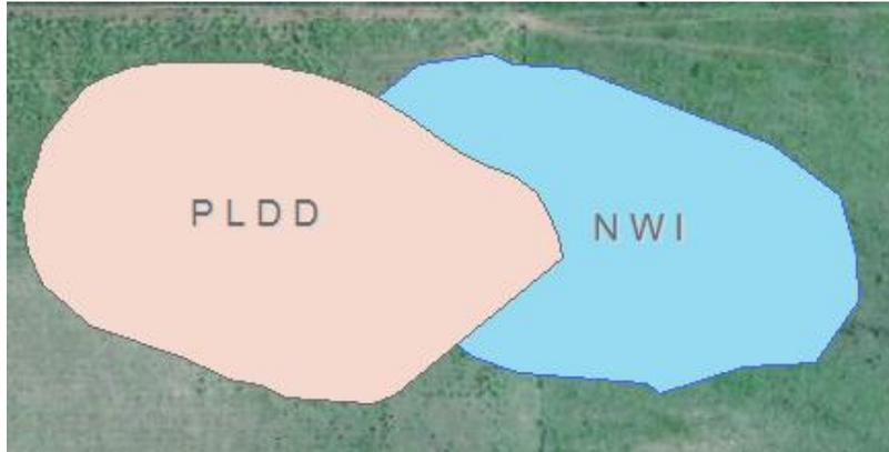
**Figure 6a. Example of a PLDD feature offset from NAIP hydric area and NWI feature by 175 meters.**
