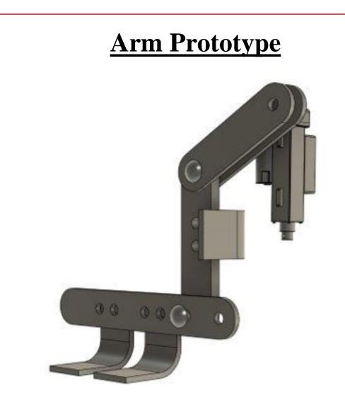
The arm's curling motion is driven using a linear actuator rated for ~200 lbf. The user controls the actuator via key fob held by the user (shown below).
