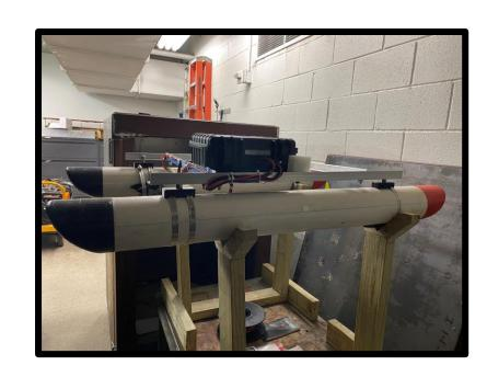
Floats are made of PVC with 3D printed hydrodynamic end caps
