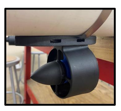
Vehicle is propelled using two Diamond Dynamics 13.1 Amp thrusters
