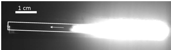
Fig. 1. Aluminum powder mixed with copper oxide powder burning in a flame tube and viewed through a 511 nm bandpass filter with a 1 nm FWHM. Note the white outline showing the tube location. The reaction was observed at 25,000 fps and 1280 \times 720 pixels with an exposure time of 10 \mu s. Image shows oversaturation region as the reaction propagates from right to left in a quartz tube.
