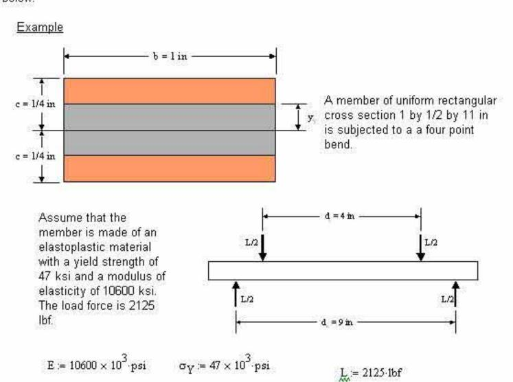
The moment from this force at the center of the beam is calculated as follows:
