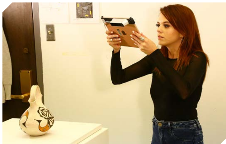
The process begins by scanning an Acoma pottery piece using an iPad & attached 3D Structure Sensor scanner.
