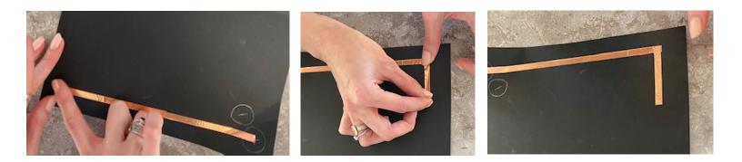
5. Leave about a ½ inch gap between the shorter copper line you just laid down and lay another shorter piece parallel towards the fold of the paper. Then lay down a longer piece that touches the end of the short piece.
