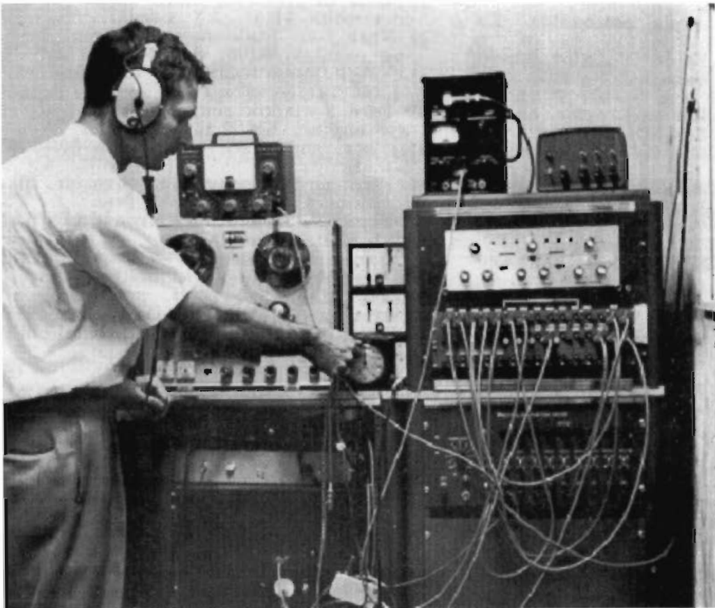
Figure 2. Bill Evans working at a panel console that could reproduce sounds for testing and analyzing reactions in humans and cetaceans. July, 1960.
