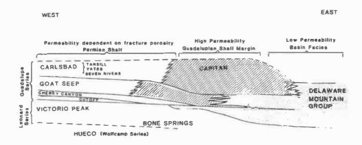
Figure 2. Permian hydrostratigraphic facies (after Nielson and Sharp, 1985). The stippled pattern denotes sandstones and carbonates overlying basinal evaporite-rich rocks; the crosshatched pattern denotes highly permeable reefal facies rocks of the shelf margin.
