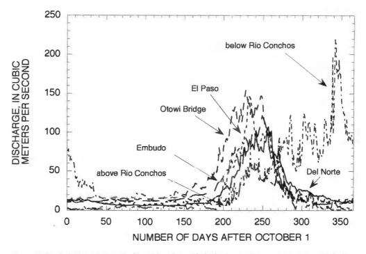
Figure 3. Graph showing median hydrographs of mean daily discharge of six gauging stations of the Rio Grande for varying periods in the late 1800s and early 1900s. See Table 2 for periods of record for each station.
