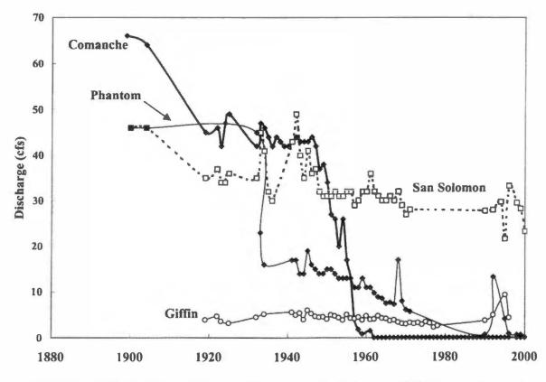
Figure 4. Spring flow hydrographs of Comanche, Phantom Lake, San Solomon, and Giffin Springs. Data are from U. S. Geological Survey, U. S. Bureau of Reclamation, and Groundwater Field Methods Class (1990, 1992, 1995, and 1996).
