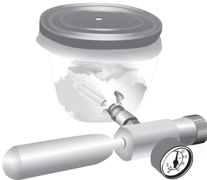
Figure 11. Illustration of a self-made carbon dioxide chamber for euthanizing a hummingbird in the field. The paper towel separates the hummingbird from the tubing that is piped into the container and minimizes the bird's access to the bottom of the container.
