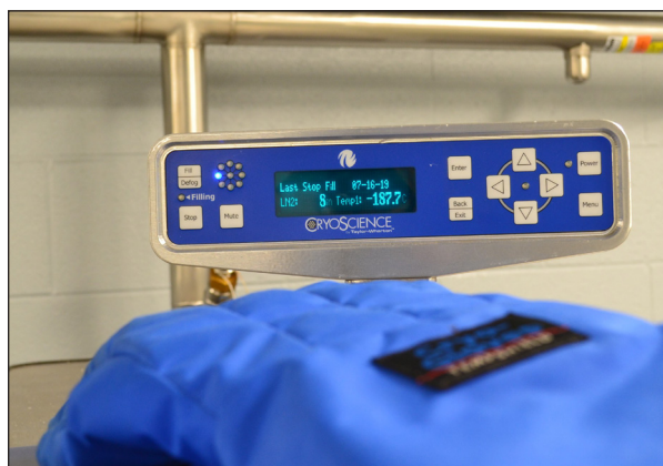
Figure 47. Controller for a liquid nitrogen freezer showing internal temperature.
