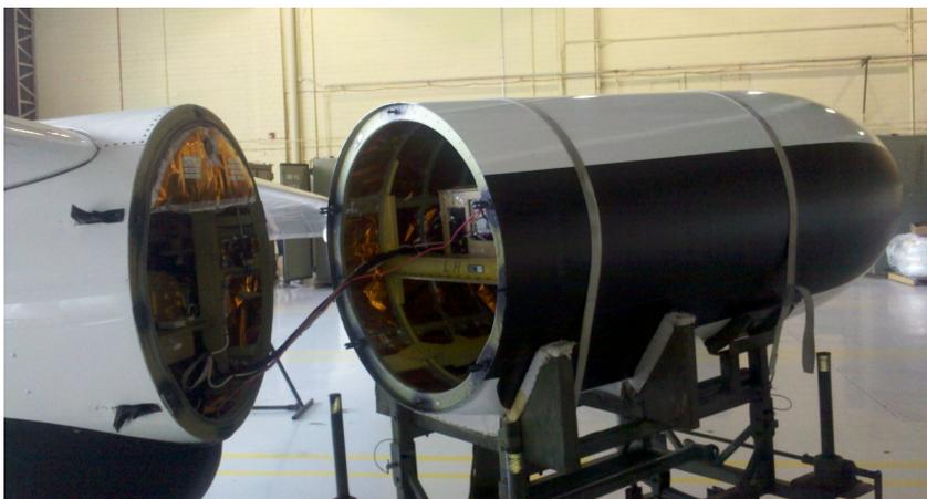
(Above) - Image of HIWRAP mounted into a wing pod on the NASA high-altitude ER-2 aircraft.
