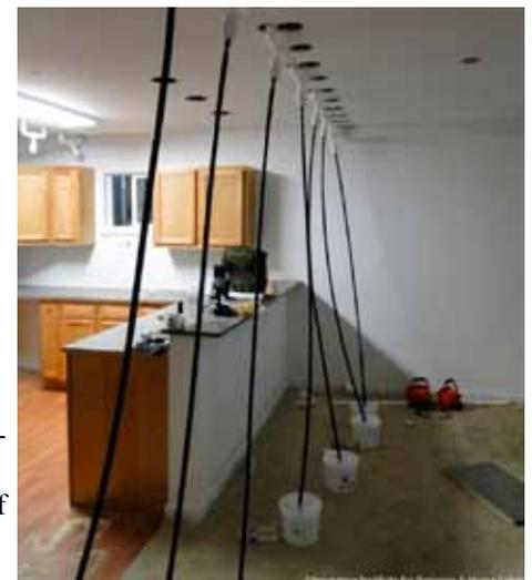
Figure 5. The water collection system located in the occupied space of the duplex test house.
