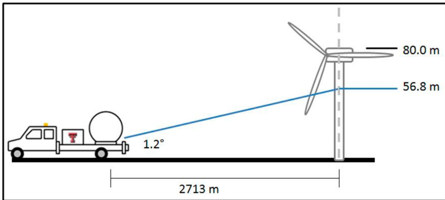
Figure 1. Schematic of the beam height from TTUKa1 at the location of the turbine based on a  $1.2^{\circ}$  elevation tilt.
