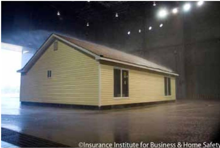
Figure 2. Wind-driven rain being blown onto the duplex test house inside the IBHS Research Center's test chamber.
