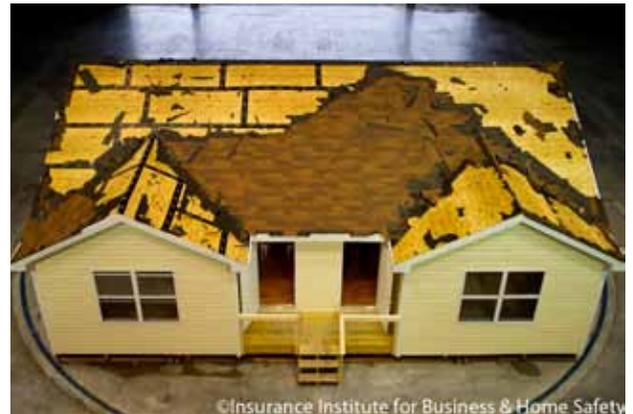
Figure 1: The duplex test house after roof shingles were blown off showing sealed (taped) sheathing joints on the left-hand-side unit and unsealed sheathing joints on the right-hand-side unit.
