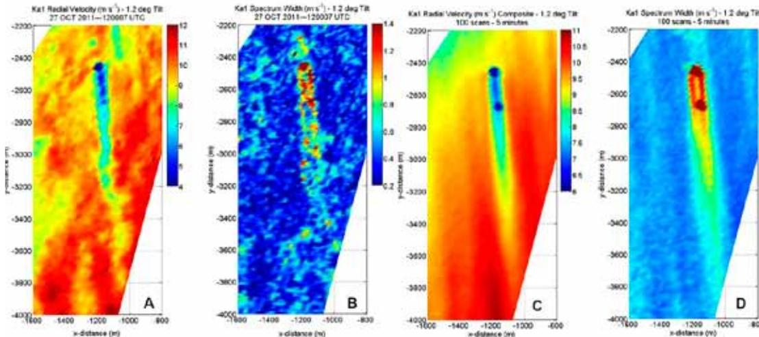
Figure 2. TTUKa1 individual PPI scan of (A) radial velocity (m/s) and (B) spectrum width (m/s). Composite fields constructed from 100 consecutive PPI scans (approximately five minutes) of (C) radial velocity (m/s) and (D) spectrum width (m/s) are also shown.
