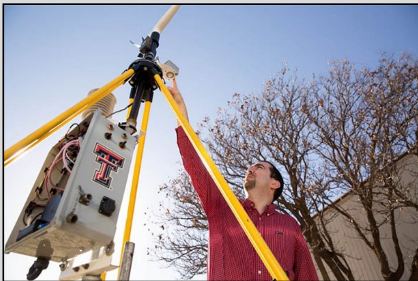
Texas Tech is using 24 mobile Sticknet platforms in the VORTEX-SE project. Sticknet is a mobile weather observation station that measures temperature, pressure and humidity near thunderstorms
