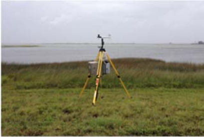
One of 24 StickNets deployed to measure a hurricane's winds and characteristics.
