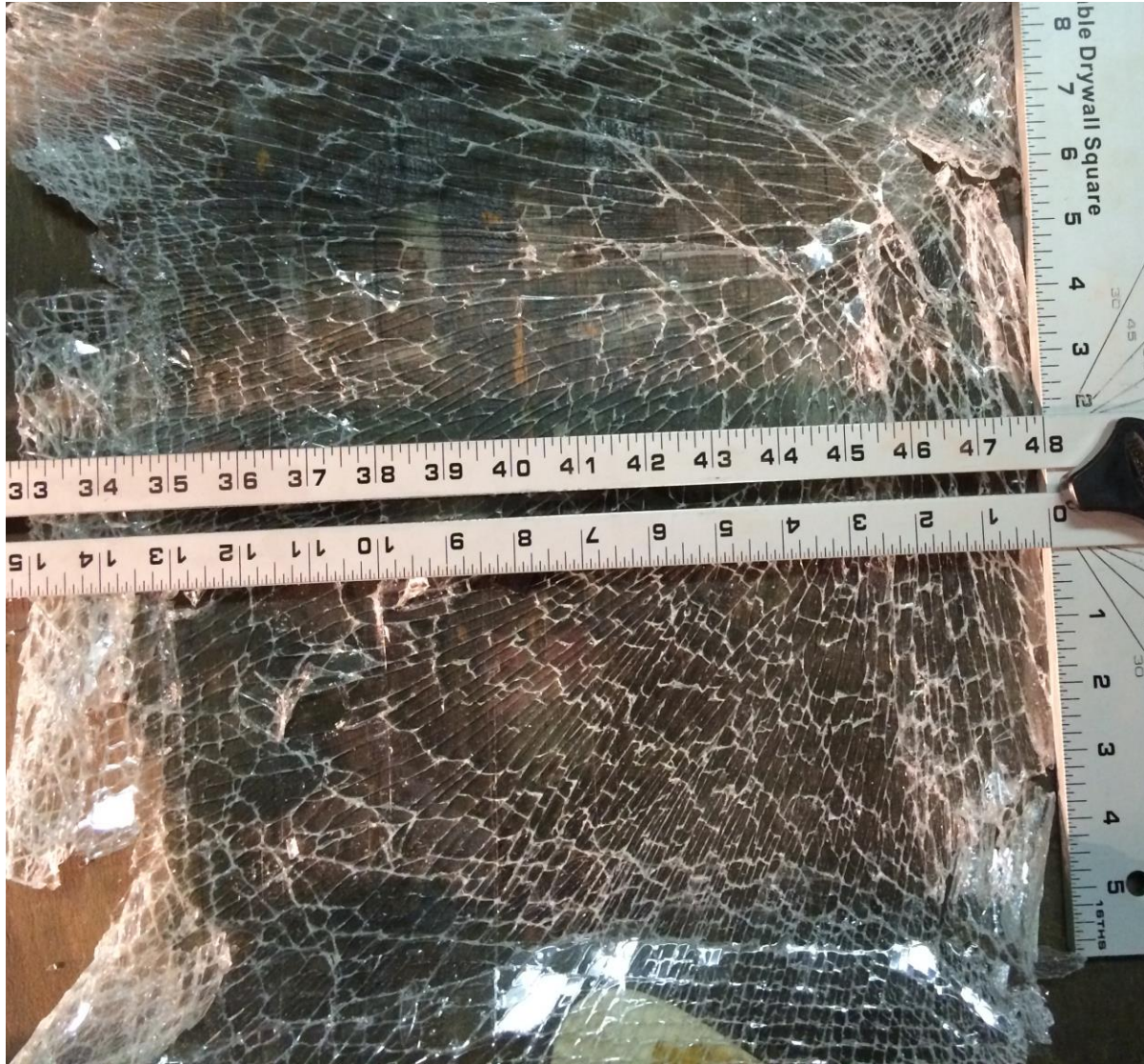
Figure. 3.2. 2.5 mm X 500 mm X 500 mm (3/32 in. X 20 in. X 20 in.) specimen loaded to failure in test lab.
