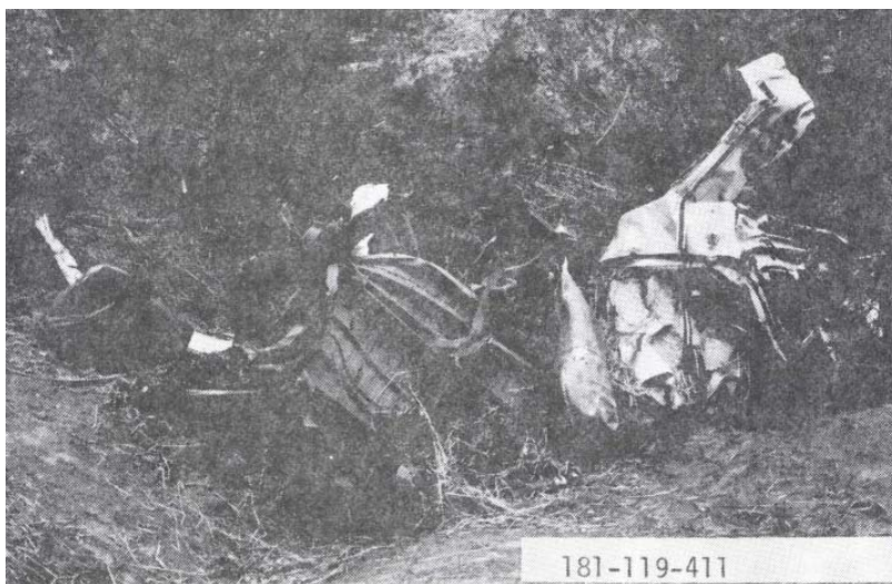
Figure 6. Remains of pickup truck. Ground marks indicated that the vehicle rolled and tumbled 500 feet.
