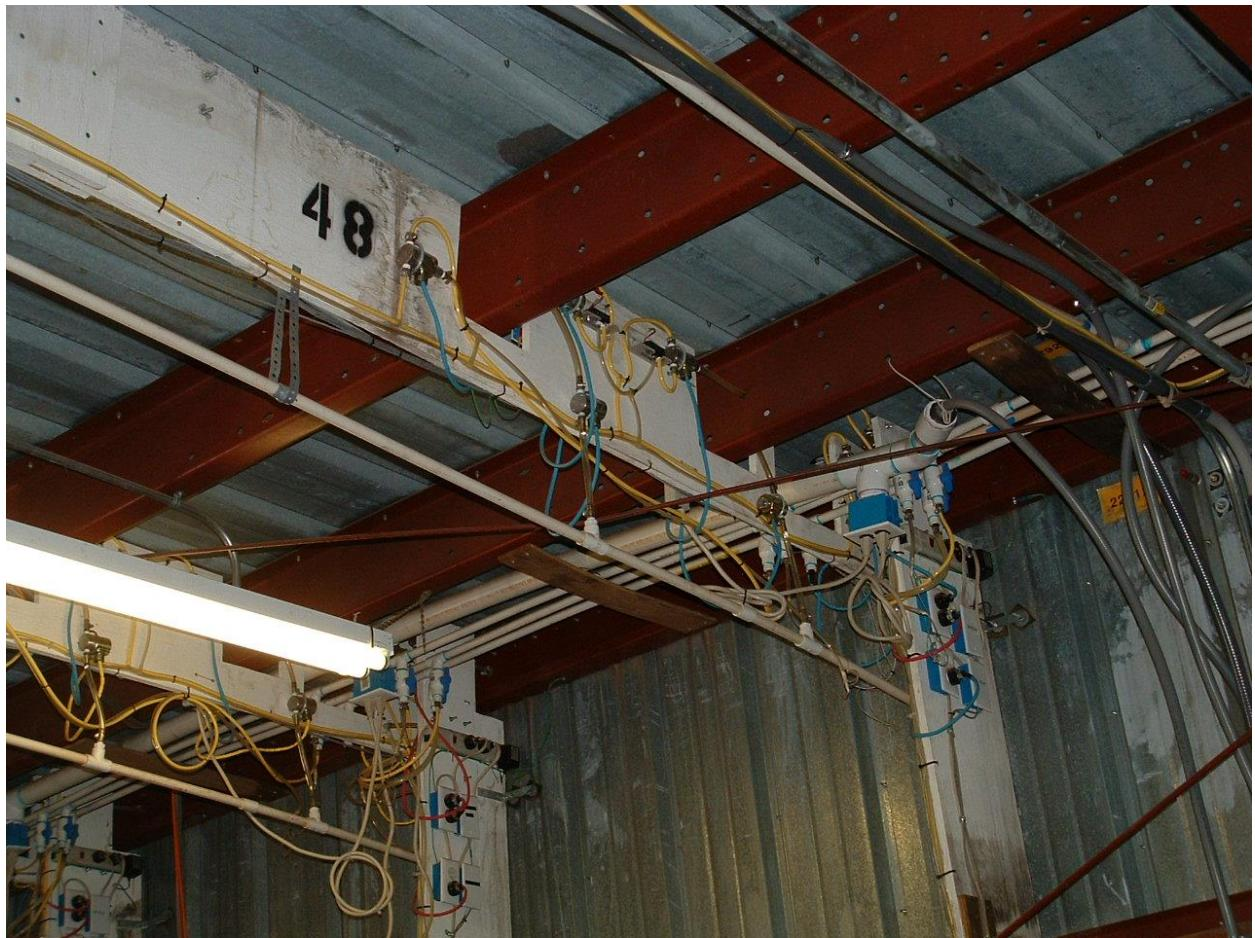
Figure 5 Organization of instruments and tubing for roof pressure measurements on the test structure.
