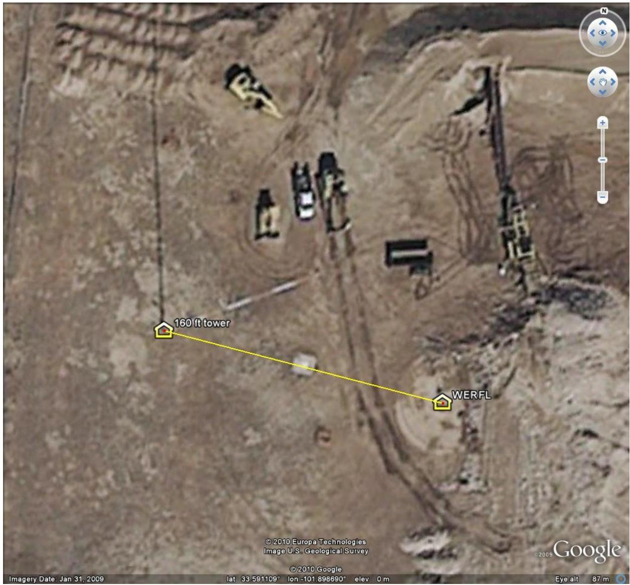
Figure 2 Orientation of meteorological tower and the test building (North is towards the top of figure and the 160 ft tower has an azimuth angle of approximately 280° relative to the center of the WERFL building location).
