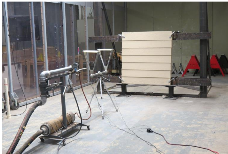
Figure 1 – Panel installation and launcher setup
