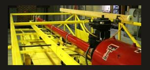
The heart of the DIF is a pneumatic cannon that plays an important role in researching effective tornado shelters for use in homes and other structures. The cannon is used to develop standards for safe above ground shelters, and continues to be in demand for testing new shelter materials and constructions.
