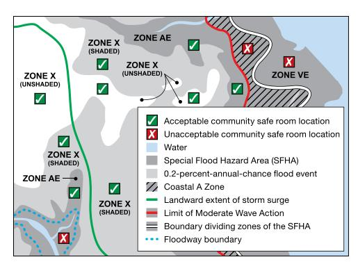
Figure B4-1. Example illustration of acceptable community safe room locations (assuming that elevation requirements are met)
