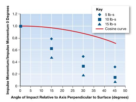
Figure B8-13. Variations of impact impulse as a function of impact angle
