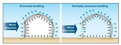
Figure B3-7. Internal pressurization and resulting building failure due to design winds entering an opening in the windward wall
