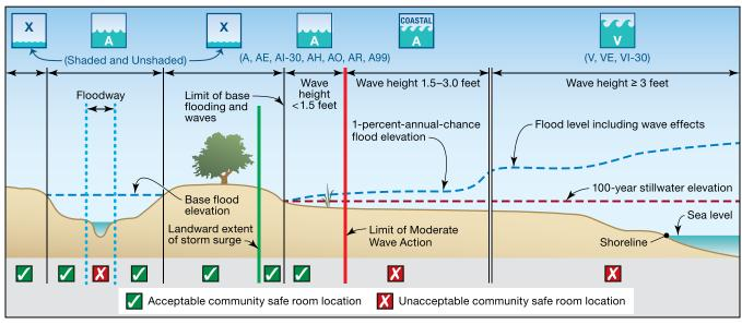
Figure B4-2. Example illustration of typical riverine cross section and shoreline transect showing stillwater and wave crest elevations and associated flood zones for acceptable community safe room siting (assuming that elevation requirements are met)
