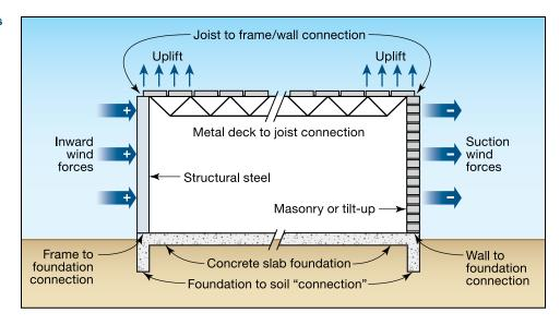
Figure B3-6. Continuous load path in a reinforced masonry building with a concrete roof deck
