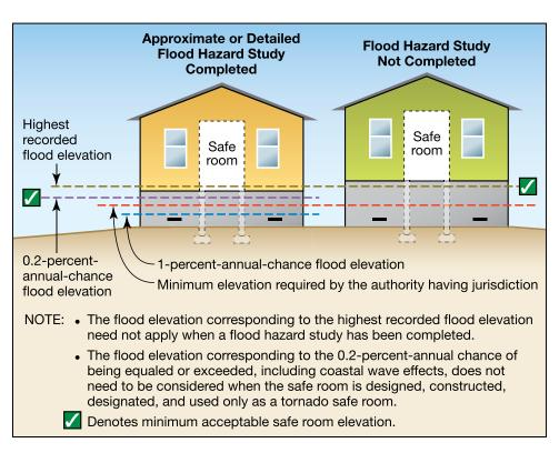
Figure B4-6. Illustration of a residential safe room example that meets flood elevation criteria (assuming siting requirements are met)
