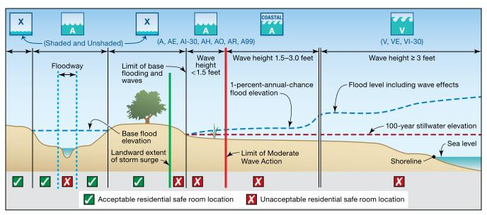
Figure B4-5. Example illustration of typical riverine cross section and shoreline transect showing stillwater and wave crest elevations and associated flood zones for acceptable residential safe room siting (assuming that elevation requirements are met)
