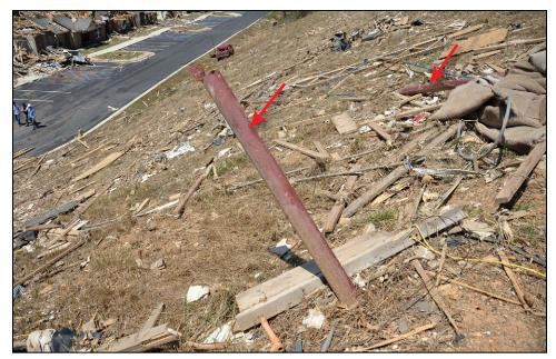
Figure B8-19. Steel porch column debris from an apartment complex where columns that were 7 feet 9 inches long and 4½ inches in diameter (see red arrows) had a significant upward trajectory and flew approximately 230 feet (Tuscaloosa, AL, 2011 tornado)
