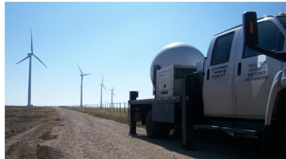
A mobile TTUKa research radar deployed at a wind plant to take detailed measurements of the wind flowing through the plant.
