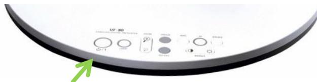
To display the PC screen again, simply turn the document camera off by pushing the power button. When the camera is off, the button turns **red**.
