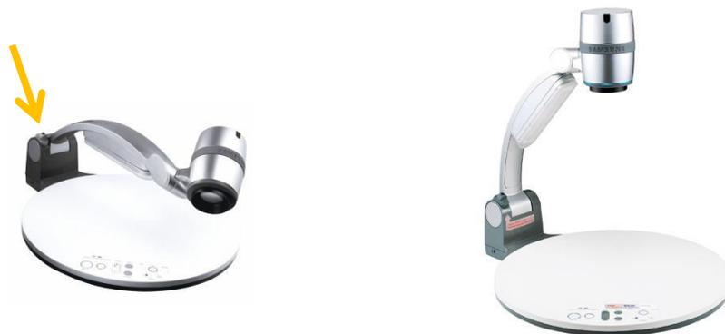
Select **PC** as the input on the control panel, and turn the camera on by pushing the power button to display your document. The power button should turn **blue** when the camera is on.
