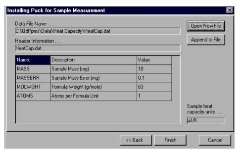
Figure 7-4. **Data File Name** panel in puck installation wizard. The name and location of the active data file are identified at the top of the panel. The information in the header of the active file is displayed below the **Header Information** box. If no data file is active, the **Data File Name** and **Header Information** boxes are blank.
