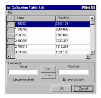
Figure 5-9. Table Displaying Puck Thermometer Resistance
