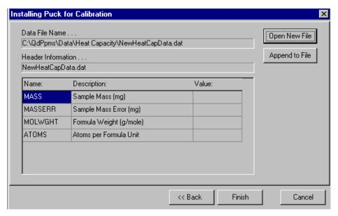
Figure 5-4. **Data File Name** panel in puck installation wizard. The name and location of the active data file are identified at the top of the panel. The information in the header of the active file is displayed below the **Header Information** box. If no data file is active, the **Data File Name** and **Header Information** boxes are blank.
