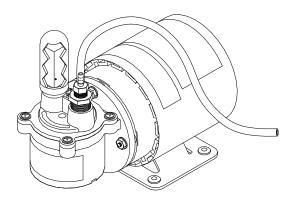
Figure 3-4. Vacuum Pump for Sample-Mounting Station
