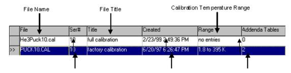
Figure 5-1. **Calorimeter Files** Dialog Box and explanation. To open this dialog, click the "Switch to New..." button on the <u>Files</u> tab.
