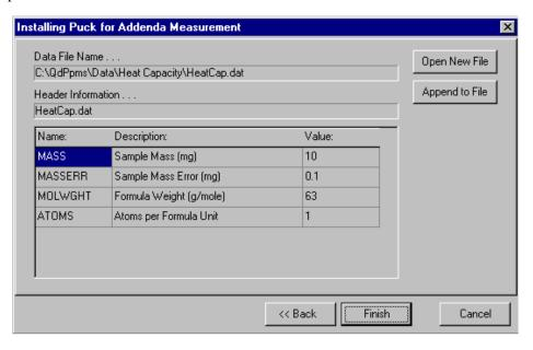
Figure 6-4. **Data File Name** panel in puck installation wizard. The name and location of the active data file are identified at the top of the panel. The information in the header of the active file is displayed below the **Header Information** box. If no data file is active, the **Data File Name** and **Header Information** boxes are blank.
