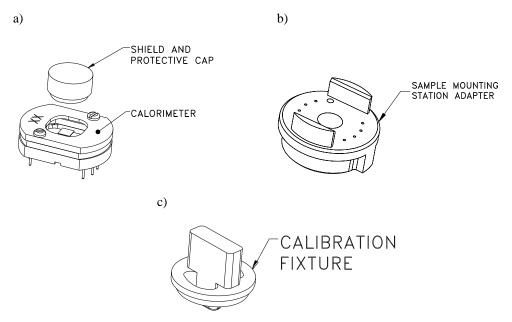
Figure 9-1. (a) Dilution Refrigerator Calorimeter puck (part number 4085-264), (b) Mounting Adapter (4092-625, and (c) Calibration Fixture (4091-624).
