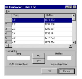
Figure 5-10. Table Displaying Platform Heater Resistance
