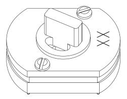
Figure 9-4. Calibration Fixture on Calorimeter Puck
