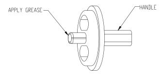
Figure 9-3. Applying Grease to Calibration Fixture
