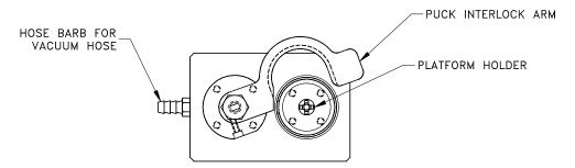
Figure 3-3. Top View of Sample-Mounting Station
