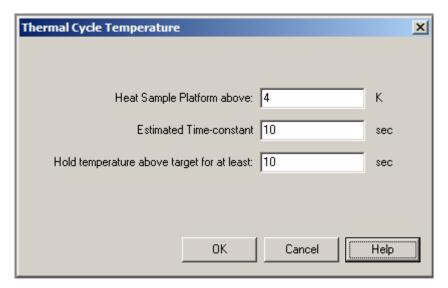
Figure 7-9 Thermal Cycle Temperature Dialog
