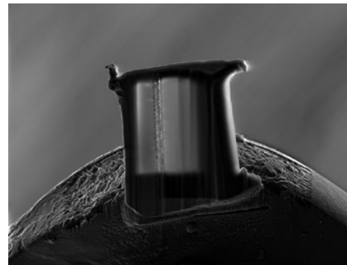
Ultra-thin TEM lamella showing interface zone on Si. Transparent area is homogeneously thin.
