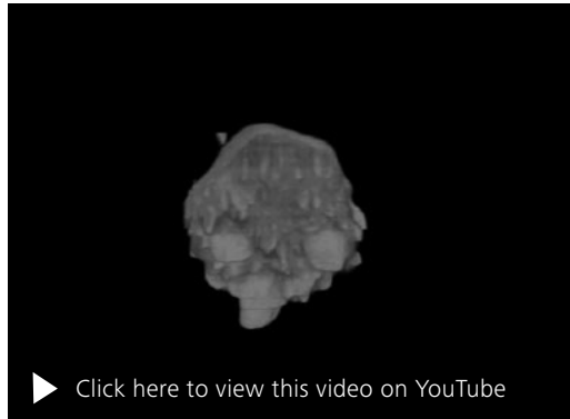
You Tube Nanocrystalline layers of silver salts of ISO 400 color film. Height: 20 \mu\text{m} ; Volume reconstruction rendered from image stack acquired in automated overnight data run.
