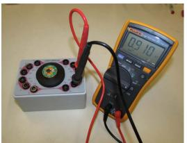
Figure 8: Checking sample for continuity
