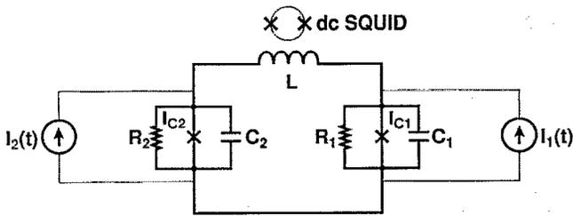
FIG. 1. The Stewart-McCumber model for two hysteretic Josephson junctions in series with an inductor  $L$ . The junctions, numbered 1 and 2, are subjected to microwave drives  $I_1(t)$  and  $I_2(t)$ , respectively. Each junction has an associated shunt resistance  $R$  and capacitance  $C$ .
