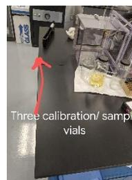
3. Place the sample in a dark cabinet to allow it to dark adapt and for any bubbles to dissipate for 1 hour prior testing. (This step can be completed inside the instrument)
