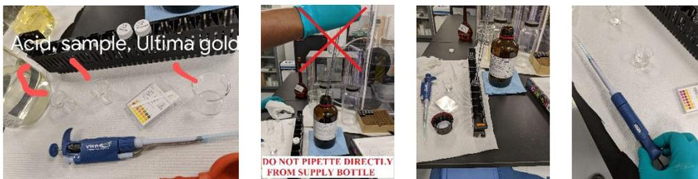
1. Measure about 10 ml of electrolyte solution to be tested into a beaker. (There should not be any particulates in the solution. Filter the solution if necessary)
