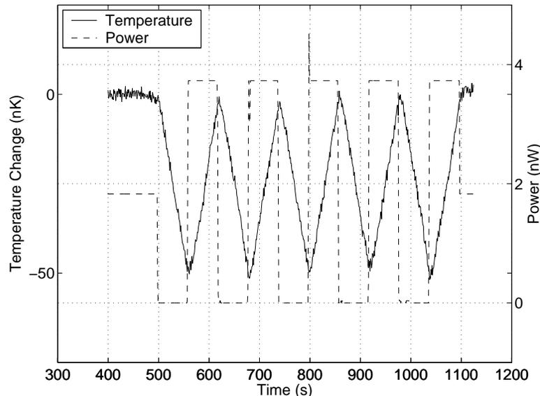
Fig. 3. Square wave biasing of the cell using Josephson array heater. These measurements were made with zero temperature change corresponding to  $120\mu\text{K}$  below the superfluid transition temperature.
