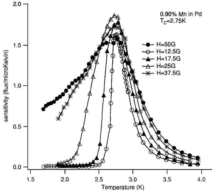
Fig. 4. Sensitivity vs. temperature in units of  $\phi_o$  per  $\mu\text{K}$  for the 0.90 atomic percent Mn in Pd sample.
