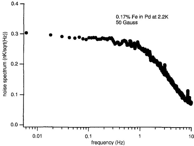
Fig. 7. Root-mean square noise as a function of frequency for the 0.17% Fe in Pd sample.
