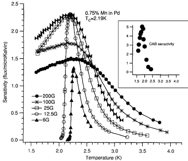
Fig. 3. Sensitivity vs. temperature in units of  $\phi_o$  per  $\mu\text{K}$  for the 0.75 atomic percent Mn in Pd sample.
