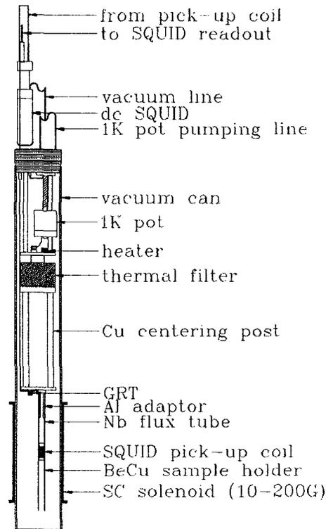
Fig. 1. Low temperature cryostat design for the sensitivity measurements.
