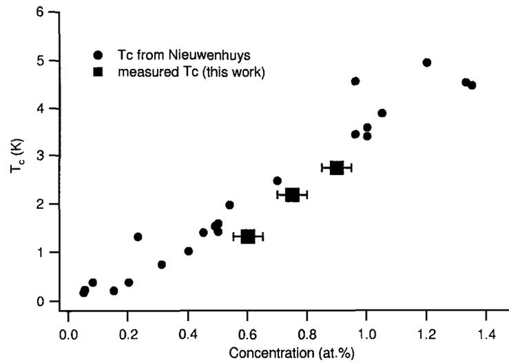
Fig. 6.  $T_c$  vs. atomic percent Mn from this work compared with that obtained by previous investigators.<sup>15</sup>
