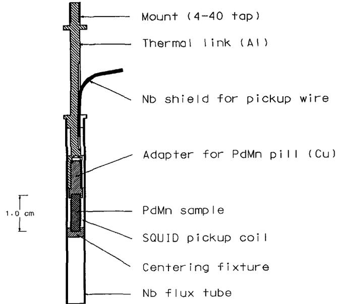
Fig. 2. Schematic of the mini-high resolution thermometer.
