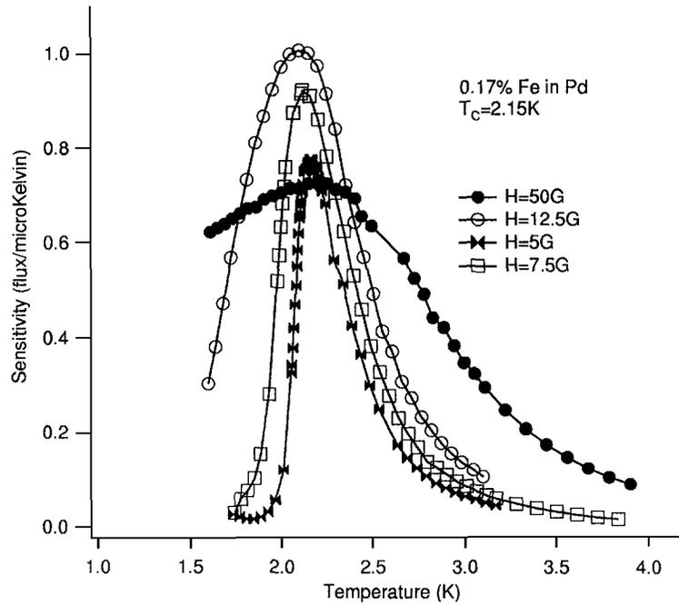
Fig. 5. Sensitivity vs. temperature in units of  $\phi_0$  per  $\mu\text{K}$  for the 0.17 atomic percent Fe in Pd sample.
