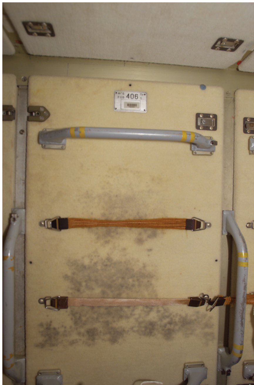
FIGURE 4.1 Microbial contaminants growing on the interior wall of the International Space Station where crew placed their clothing after working out. The panel eventually had to be replaced after attempts at decontamination failed. SOURCE: NASA Image ISS010E11563, available at http://www.nasa.gov/mission_pages/station/science/experiments/Environmental_Monitoring.html#images .
