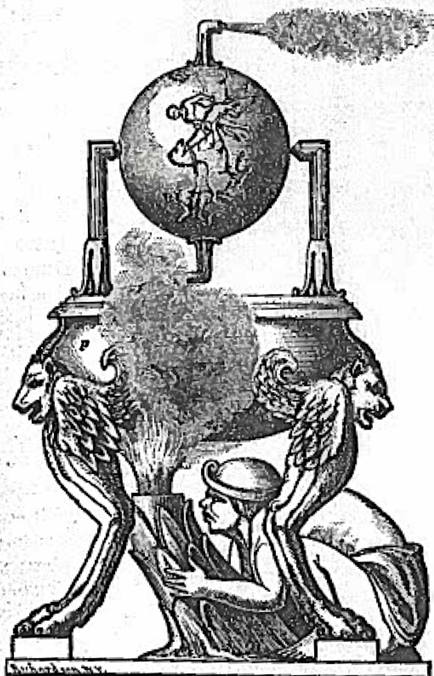
FIG. 1.—THE GRECIAN IDEA OF THE STEAM-ENGINE.
