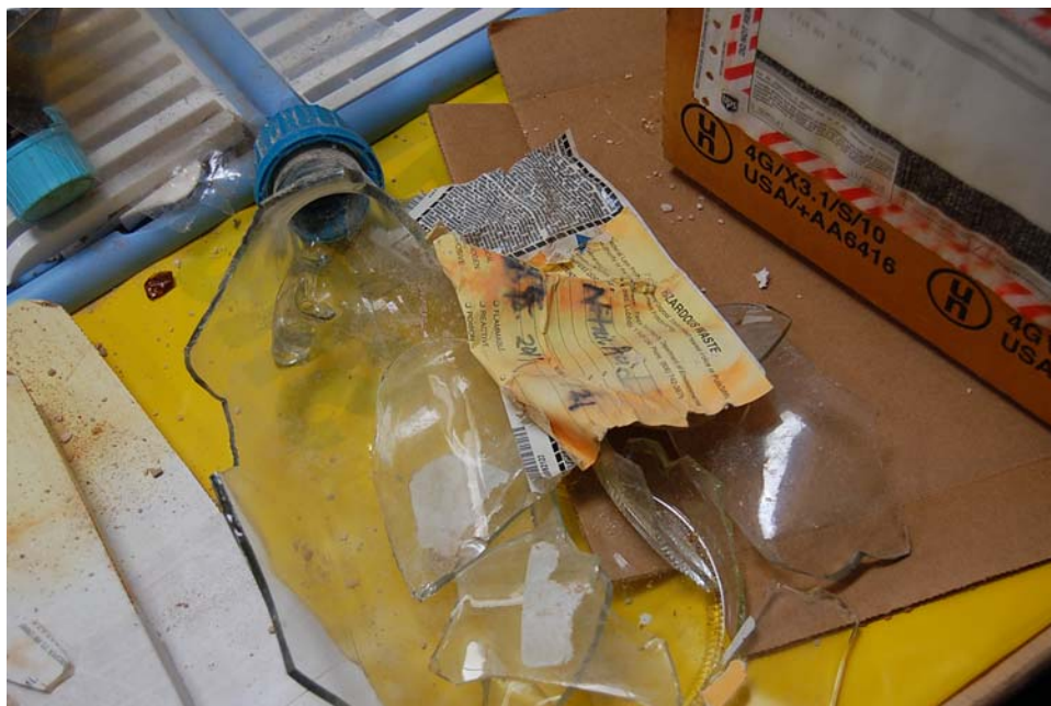
Image 7. 4 liter bottle of Nitric acid waste that was broken.
