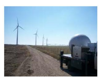
National Wind Institute researchers developed a new <u>radar system</u> capable of measuring wind flow within wind energy plants.
