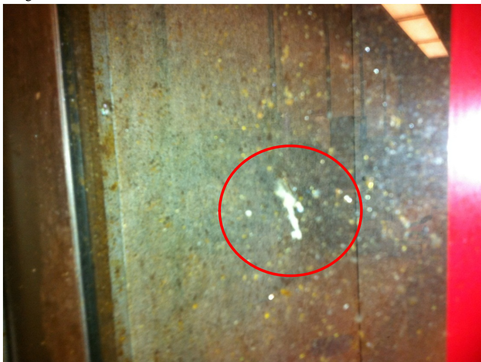
Image 10. Strike mark on fume hood sash where it is cracked.
