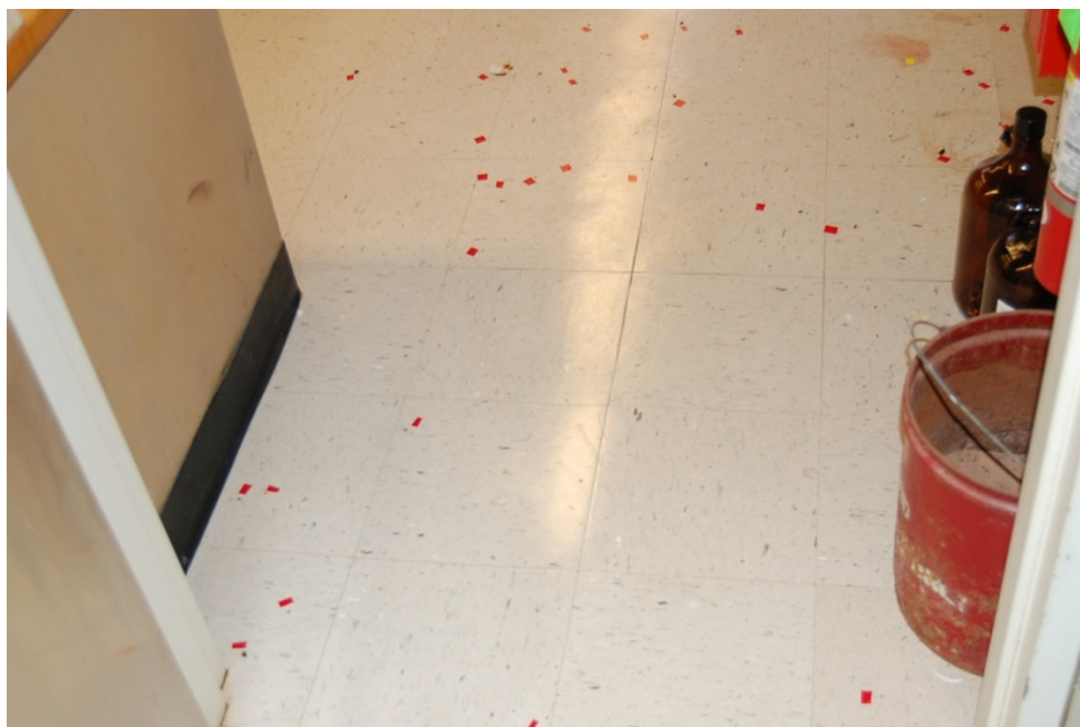
Image 3. Floor of laboratory approximately 56 feet from incident. The red marks are where amber glass shards were located.
