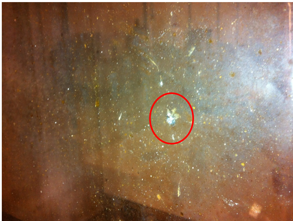
Image 9. Strike mark on fume hood sash where it is cracked.
