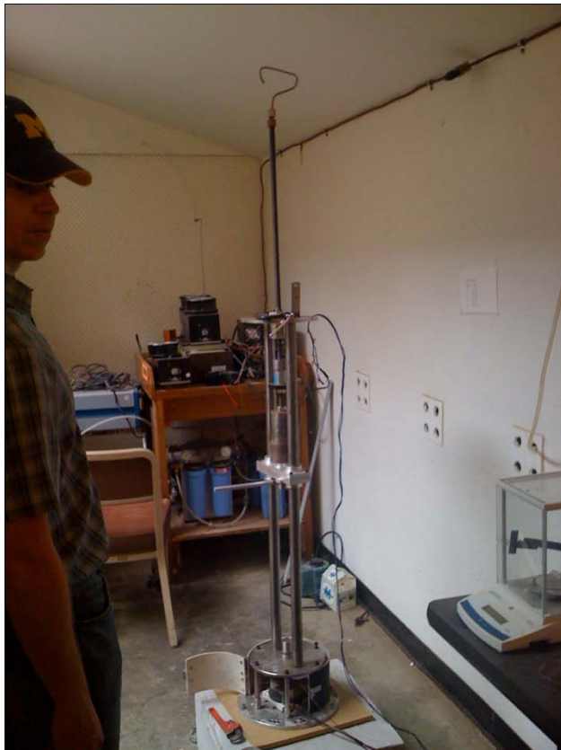
Figure 2. Drop-weight impact test device set up in an isolated area in the Prof. Brandon Weeks' Room 6 laboratory.
