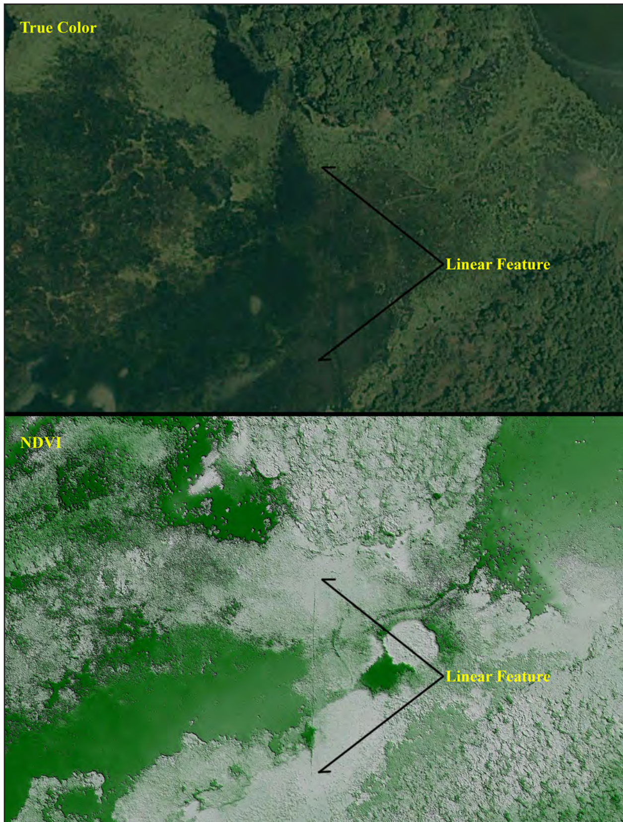
Figure 5.9. Linear anomaly in Laguna Seca invisible in the visual spectrum (top) but clearly identifiable in the custom NDVI data (bottom).
