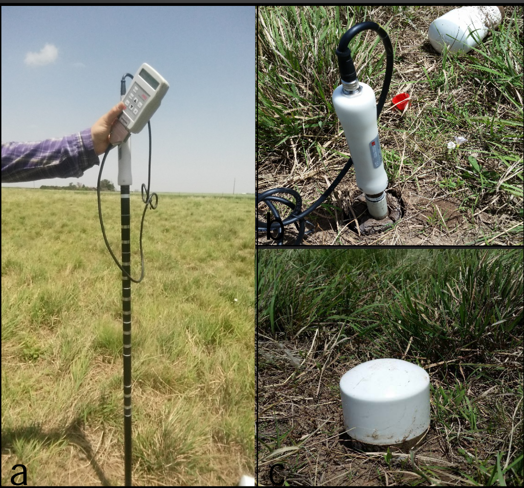
Figure 2. Capacitance probe (a) is inserted into access tube (b) for rapid VWC reading. PVC covers provide protection (c).
