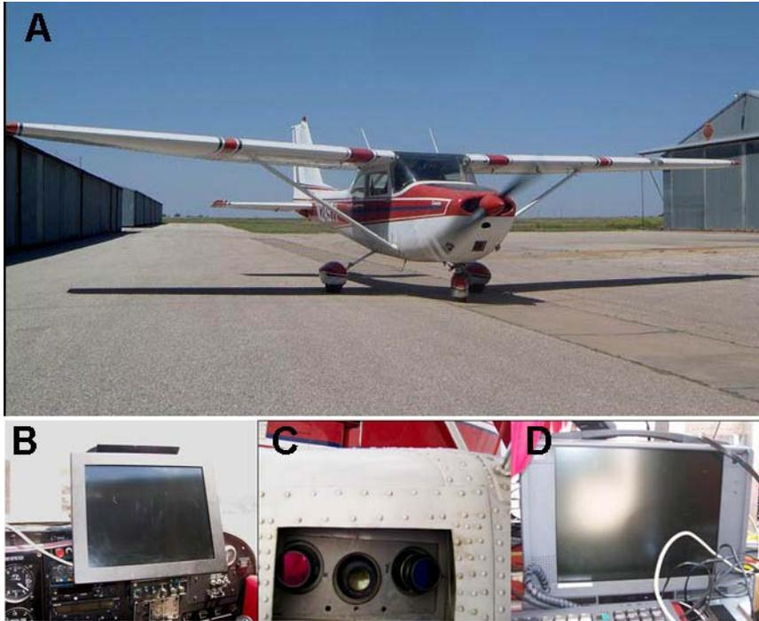
Figure 13. Components of TTAMRSS. (A) Cessna Skyhawk aircraft; (B) System monitor; (C) View of underside of aircraft showing cameras; (D) computer.
